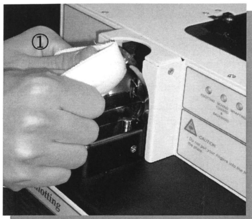
将扣子放入插座之间 Put the button in between the slot.
